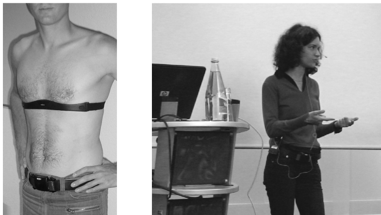
Fig. 3. Wearable system used for the recording of heart period data during the conference session. Left: Heart monitor belt attached to the thorax and QBIC belt computer for data storage. Right: Speaker wearing the system during the conference talk.
